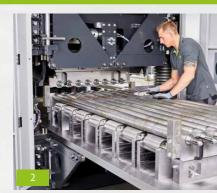
The advanced cleaning system makes it easy to clean the leveling rollers and supporting rollers using the fully extendable leveling cassette.
