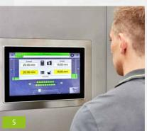
The intuitive user interface speeds up the process of entering settings for different materials on the part leveling machine. A state-of-the-art multi-finger touch display lets the machine operator enter, save, and reload settings.
