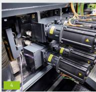
The direct drive brings many advantages: greater energy efficiency, less wear and reduced noise, greater machinable profile, material processing while protecting the surface, and higher torques transmitted to the leveling rollers.
