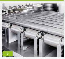
Extra-wide supporting rollers provide extremely stable support for the leveling rollers over nearly 50% of their length. The benefits: Extremely precise concentricity, higher power input, less wear, and reproducible leveling results.
