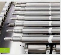
Patented reversible leveling rollers increase the service life of the rollers when leveling narrow parts on machines that have a comparatively large processing width.
