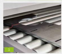
**Return feed operation** allows the machine to be loaded and unloaded from one side. After the leveling process, the top roller frame will automatically open, change the rotating direction of the leveling rollers, and send back the material.
