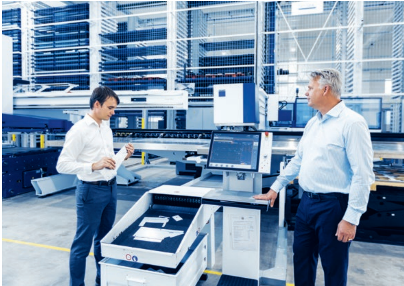
Switchover: The software monitors production and maximizes utilization of the sheet metal to avoid scrap.
